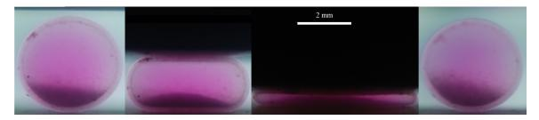
**Figure 5:** Example of compression of a capsule of diameter 3.7 mm and a membrane thickness that is 10 % of radius, shown at 4 points during the compression. The capsule has been coloured red and time progresses from left to right. Note that the capsule returns to its original shape after the compression.
